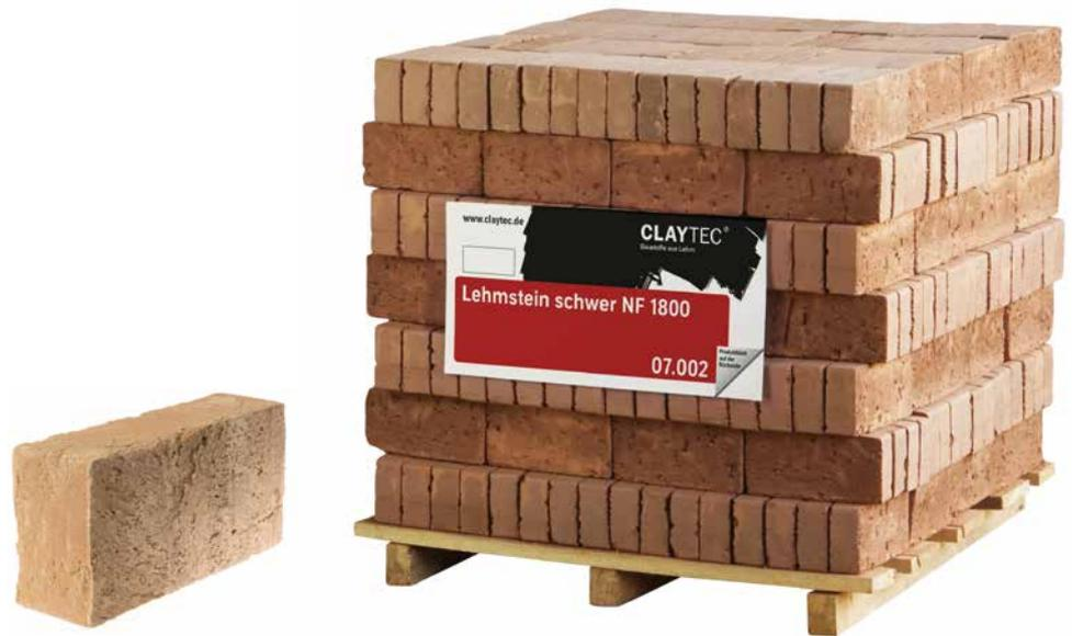
Mould-made clay block of application class Ib (= approved for load-bearing walls). Can you build load-bearing walls with clay? Yes, with the clay block 1800 NF. 30 years ago, CLAYTEC developed this block, which is unique on the market. The normal format (NF) makes it particularly suitable for small-scale repairs of historic solid clay buildings. Heavy clay masonry mortar is suitable as a mortar.
