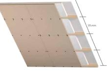
Drywall board made of clay and reed for cladding of wood and metal post structures of inner walls, facing shells, ceiling and roof surfaces. Claytec Clayboard acts both as drywall board and clay plaster. It was created based on manual experience and has been on the market for over 20 years. With a bulk density of 700 kg/m<sup>3</sup> it offers clay mass and is easy to handle. As supplement to this product sheet the **CLAYTEC Guidelines for ecological drywalls in system apply**.
